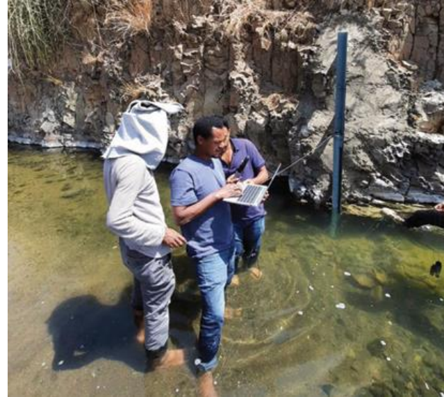
Establishing a flow gauging station in Ethiopia
